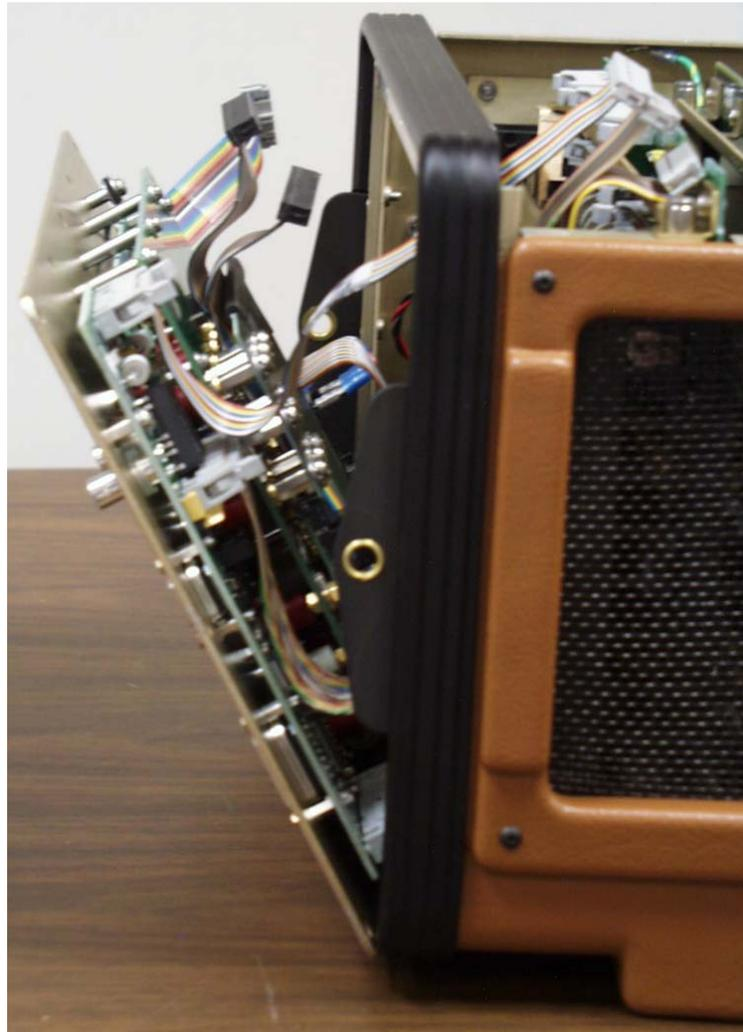
*Figure 7.4 Instrument Front Panel Tilted Forward 30°*
