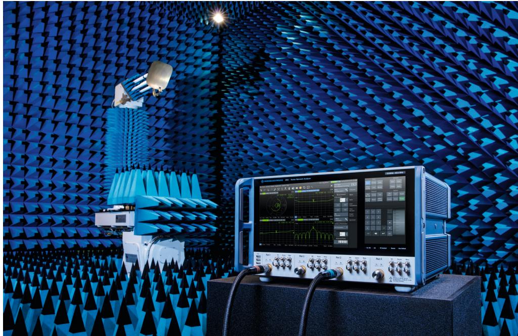
Figure 22: R&S®ZNA used for antenna measurements
