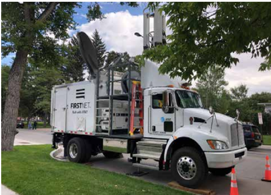
A FirstNet-AT&T SatCOLT, a Cell on Light Truck deployable that uses satellite-based backhaul.
