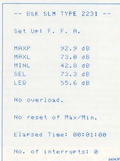
Fig. 6. Printout from Type 2231 with Module BZ7100, Graphics Printer Type 2318 and Interface ZI 9101
