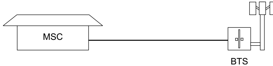
Figure 8-2. One Possible T1 Network Topology
