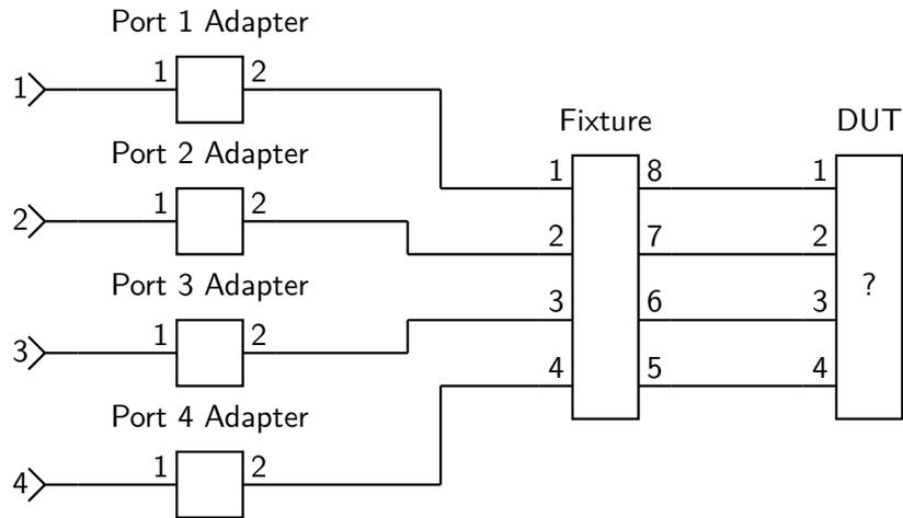
Figure 4: Fixture and adapter de-embedding circuit
