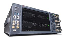
Nonlinear measurements of the array, such as swept gain compression and error vector magnitude (in the classic "bathtub curve" of EVM vs. power), are made by driving the device into compression. The VXG-C provides a wideband modulated signal through a booster amplifier. The PNA-X also supports the Keysight PathWave Vector Signal Analysis software if other demodulation metrics like error summary tables, spectrum and time displays, and constellation diagrams are needed.
