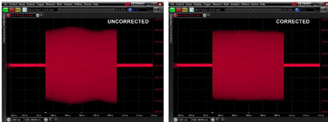
Figure 10: The effect of applying corrections can be seen in this pair of scope screen captures. The signal shown is a 4GHz chirp on a 10 GHz carrier. Improvement in pulse flatness is impressive. The same kind of improvement can be achieved for radar signals using polyphase modulations (i.e. Barker or Frank codes), where EVM improves dramatically.
