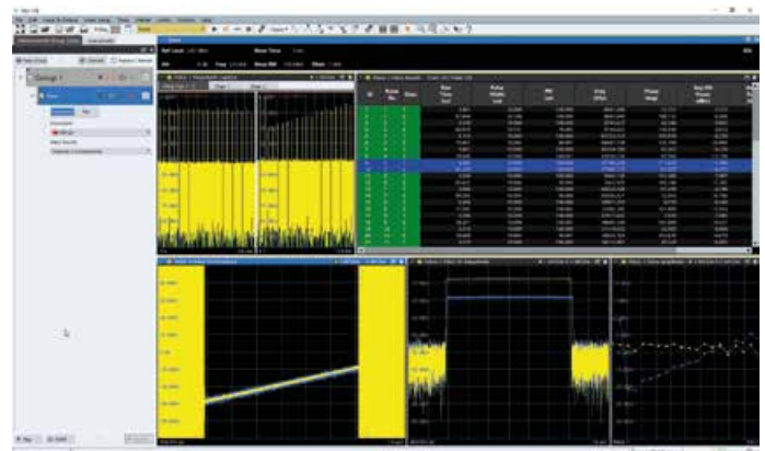
Fig. 3: In-depth analysis of the retransmitted pulse echo (channel 3) in relation to the original pulse (channel 1) with the R&S®VSE-K6A multichannel pulse analysis option
