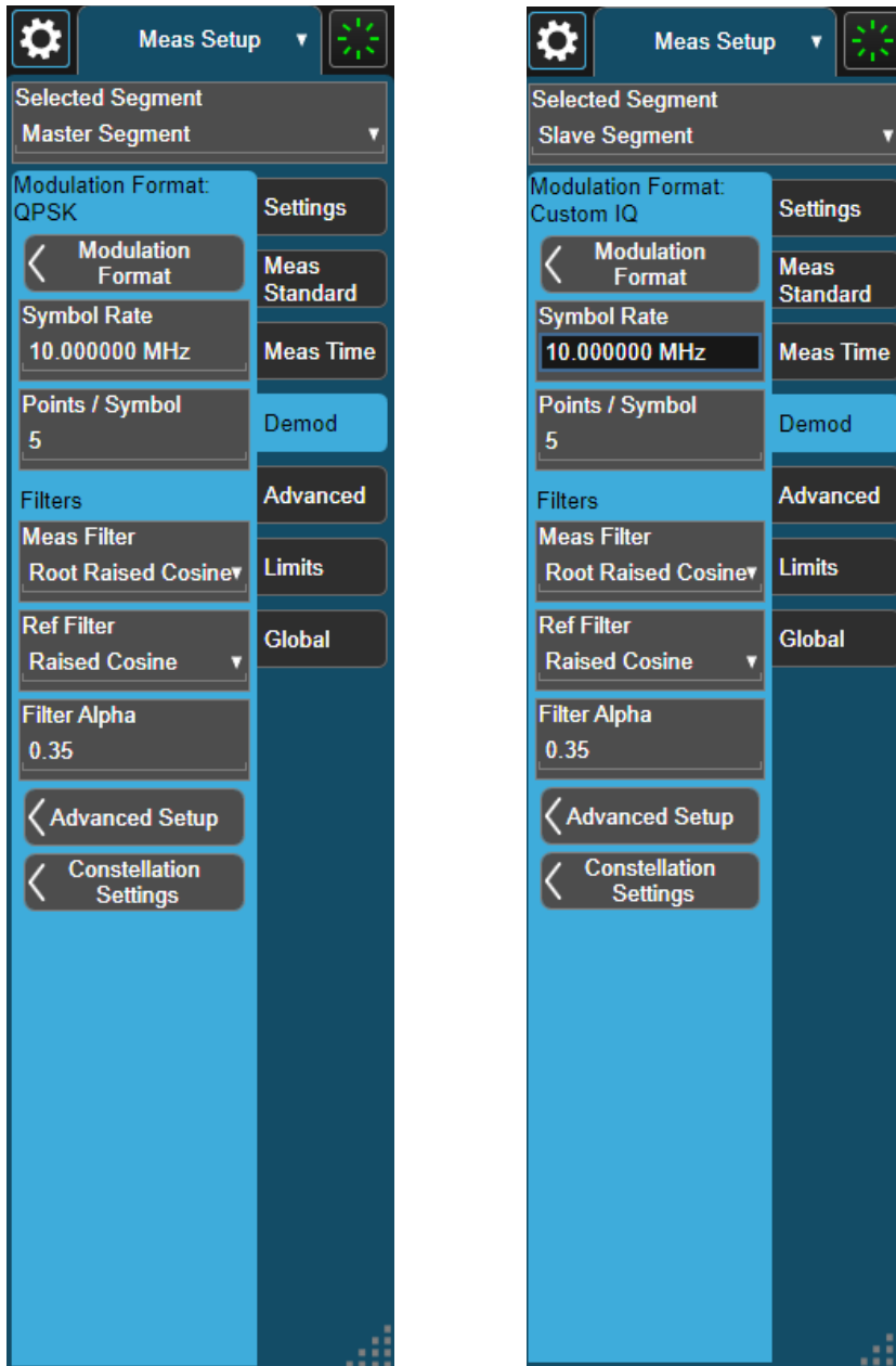
Figure 3. Parameter setup for primary and data segments for demodulation
