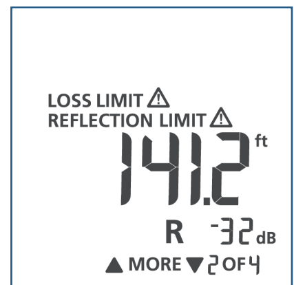
Figure 3. Depiction of a Fiber Troubleshooter showing reflection and loss limits exceeded.
