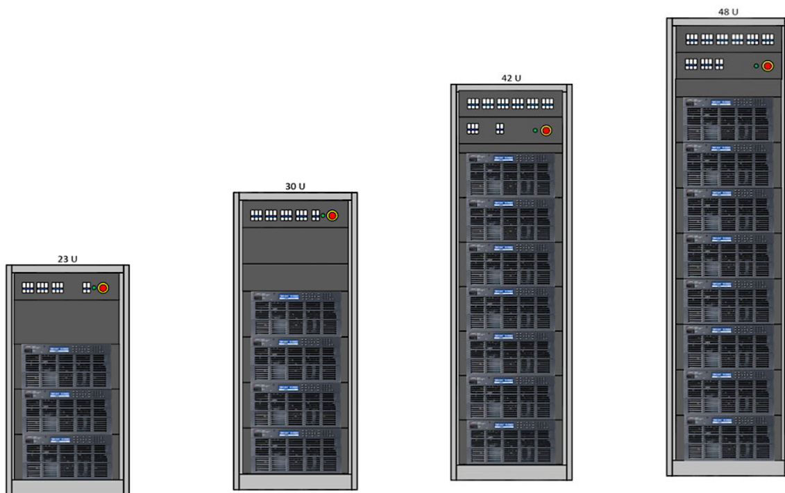
Figure 1. Rack setup, from left to right: 90 kW, 120 kW, 210 kW and 240 kW
