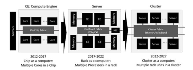
The second phase of enhancing compute throughput, observed between 2017 and 2022, involved treating a rack as a compute unit by connecting multiple rack units in a cache-coherent manner. During this period, machine learning applications began to take shape in compute clusters organized as data center networks, with server racks serving
